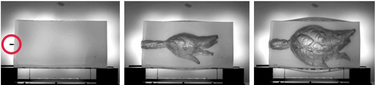
**Figure 4.16.** .308W 175gr **Hollow Point (HP)** projectile. Left: Prior to penetration of the projectile; Middle: Initial expansion; Right: Final expansion.
