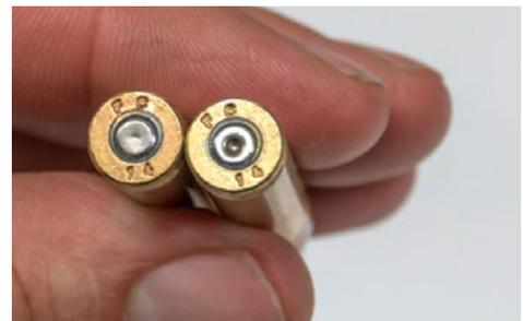
**Figure 4.18.** A centrefire cartridge showing light primer strike on left, normal strike on right.
