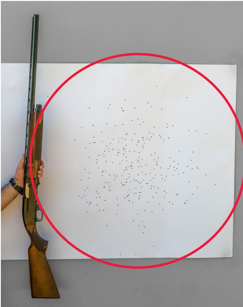
*Figure 6.3. Shotgun pattern – modified choke at 20 metres.*
