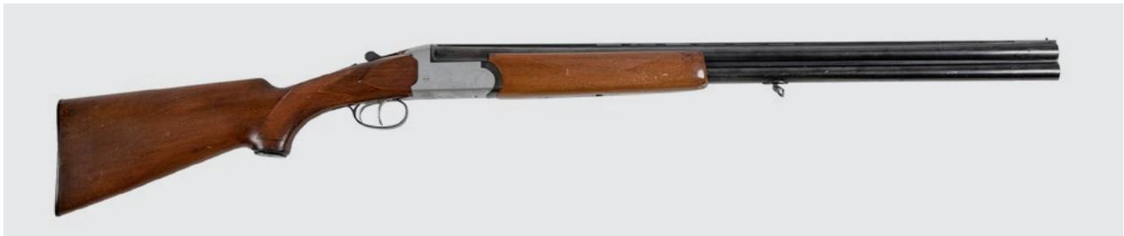
Figure 3.6. Double-barrel over-and-under break-open shotgun.
