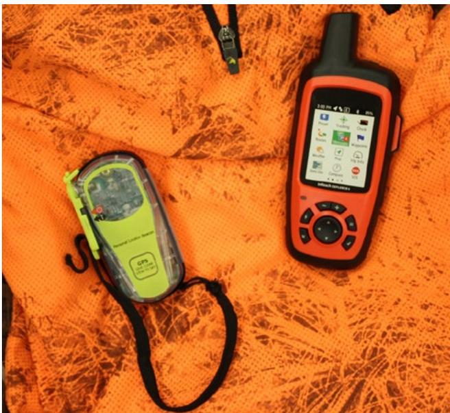
Figure 8.3. PLB on left, GPS on right.
