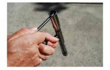
When shooting is finished, remove the bolt from the action, replace the bolt key onto the rear of the bolt and rotate back to the unloaded position.
