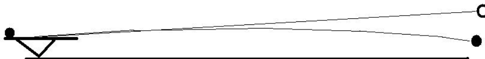
Fig 3 Open circle is the image of the target the shooter sees when the air is calm and the mirage is boiling
