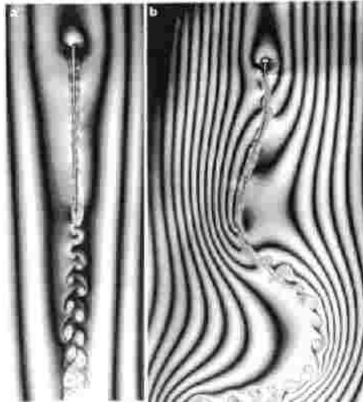
The photos depicts the flow around the flag. (a) steady, (b) in the flapping stage.
